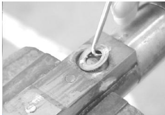
Figure 8.2: Remove and discard the copper washer.
