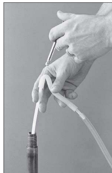
Figure 17: Syringe sampling for field analysis.
